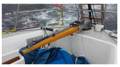
its NMEA 2000 networks, we were finally able to sail with the Autohelm on apparent wind or true wind. This is a must for keeping the boat going fast, especially if you need to get some rest.
